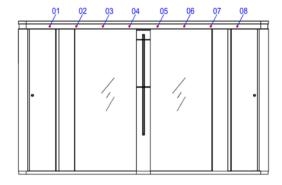
The PG500 with 1600mm cabinet is fitted with 8 high level transmit / receive detection sensors as standard (top row 01 to 08).
