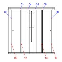
fitted with 6 high level transmit / receive detection sensors as standard (top row 01, 03 to 06 and 08).
