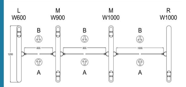
Single leaf arm standard widths are 550mm, bespoke options from 500 to 550mm are available on request.
