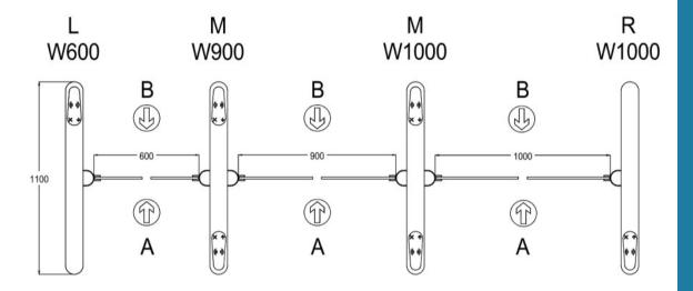
Single leaf arm standard widths are 525mm, bespoke options from 500 to 525mm are available on request.
