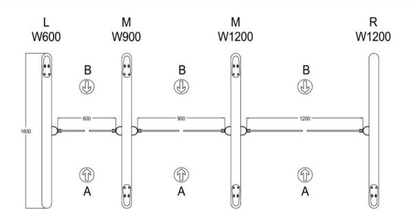
Single leaf arm standard widths are 600mm, bespoke options from 500 to 600mm are available on request.
