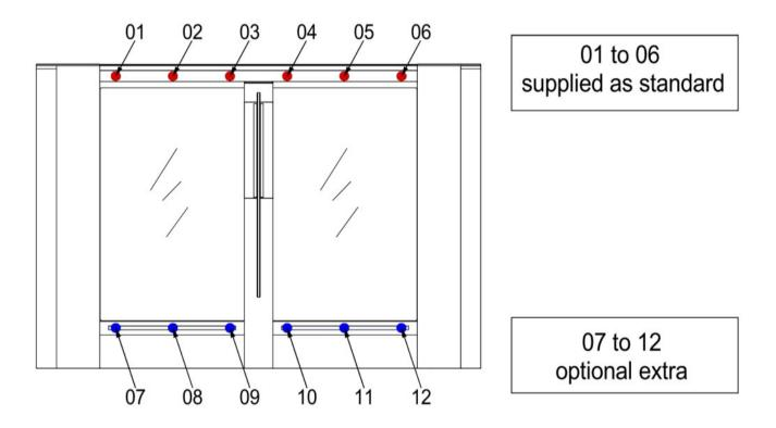
As standard the PG127 is fitted with 6 high level transmit / receive Omron detection sensors to monitor and protect the control zone.
